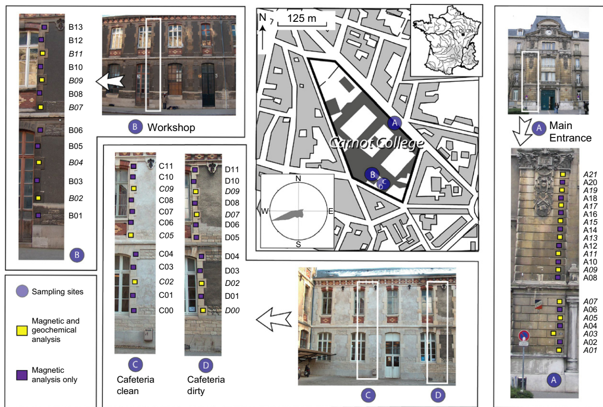
Fig. 1. Map of Carnot College, Dijon. The blue spots represent the targeted façades: ‘Main entrance’, ‘Workshop’, ‘Cafeteria/clean’ and ‘Cafeteria/dirty’, on which in-situ and laboratory magnetic susceptibility and geochemical analyses (yellow boxes), or only magnetic analyses (blue boxes) have been performed. Sample codes are shown to the right of the façade close-up. The main wind direction when it rains in Dijon (> 5 mm) is also indicated. In Dijon, the mean annual temperature and the relative humidity are about 10.7 °C and 71%, respectively. All calculations have been performed on the basis of the 1971–2000 record. (Meteo France, pers. comm., 2007).
