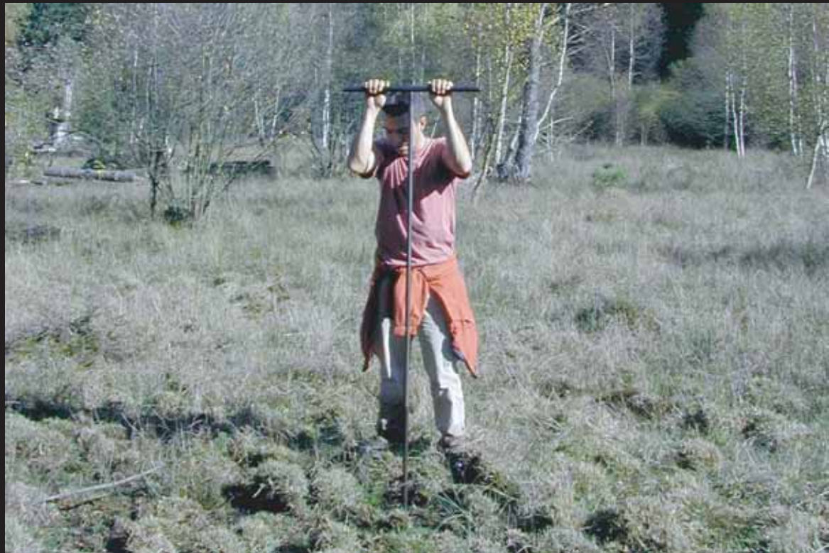
Fig. 2: Sampling with GIK-type corer
