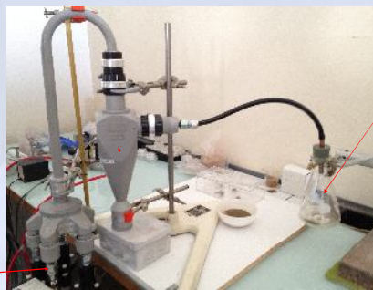
10 µm cut-off cyclone
