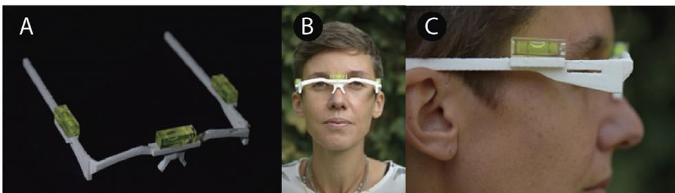
**Fig. 2.** The prototype ensuring the horizontality of the reference plane on both axes. A: the mount with bubble levels; B: an example of use; C: the slot on the side of the frame allows the eyes to be aligned.
